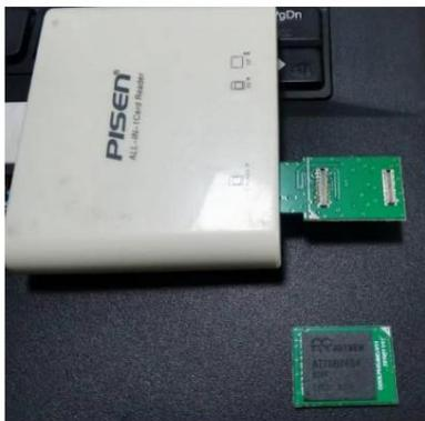
If it is not easy to insert into the card reader, grind the edge or cut it off with a knife and then insert it into the card reader
