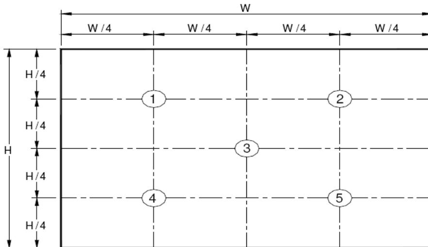
Figure 8. White Luminance and Uniformity Measurement Locations (5 points)
