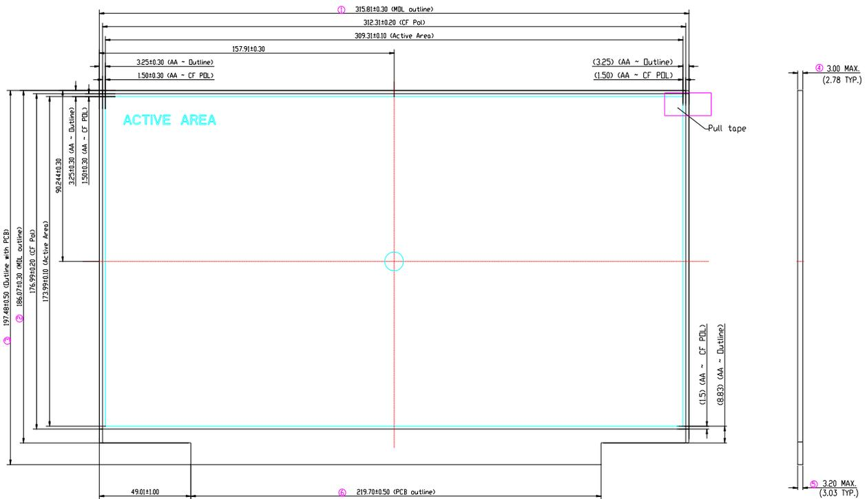
Figure 24. TFT-LCD Module Outline Dimension (Front View)
